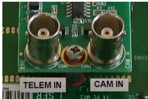
Video Connections controller and camera
