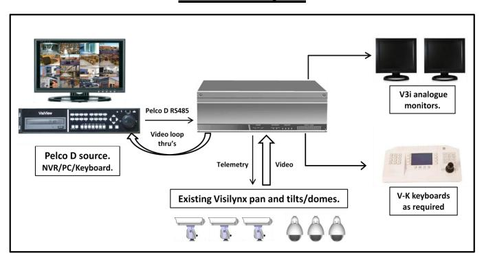
The Pelco D source is connected to a 9 way d-sub communication port on the rear of the V3i matrix, loop thru's take video from the V3i to the Pelco D source. View and control your existing Visilynx cameras via the internet.
